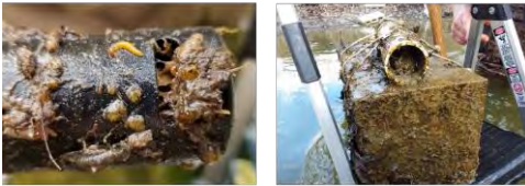
Figure 3.9 Examples of Fouling Observed on CTD-10 Sensors
