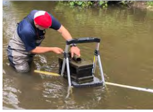
Figure 3.8 CTD-10 Sensor Cleaning and Maintenance
