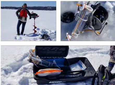
Figure 3.16 Equipment Used for Winter Lake Sampling
