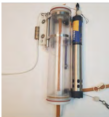
Figure 3.14 Niskin-Style Vertical Water Sampler and Aqua TROLL 500 Multiparameter Sonde Assembly
