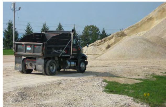
Having sources of aggregate relatively close (within 25 miles) of a construction project lessens the overall cost of construction due to the cost of transporting heavy materials.
